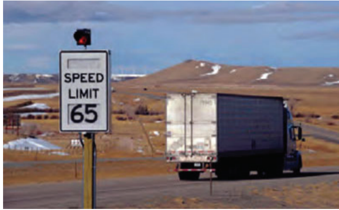
Variable speed limits can decrease traffic speeds in adverse conditions. | Photo credit: USDOT
