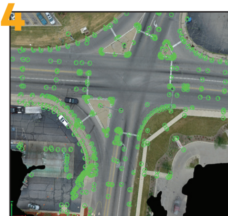
4. The "Virtual Survey" of the crash scene is depicted. Instead of using a Total Station or tape measure, the green dots are points to create a diagram. The point list is the excel file at right (5).
